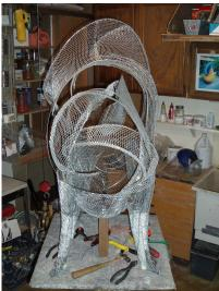
This shows additional jigging on the front side, along with a support for the bottom.
