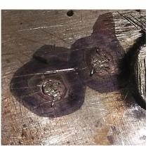
The fourth shows the result of this welding after grinding the surface. Neither weld was successful because the pellets were not large enough to fill the pits and small pitting and rings around the welds are visible. The fifth shows the two pits (still about .020" in diameter ) re-welded with pellets 0.40" in diameter. The sixth shows the results of this welding after grinding and re-prepping. One of the welds was dirty and deeper than expected and required another welding session. 5 6 4
