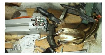
To weld, pressure is applied to the pellet or filler material with the tip and power is applied. For small pellets, power is adjusted by using fewer of the bottom cables and/or clamping the bottom cable farther from the weld point and/or using the extra piece of cable. Adjusting duration of the power cycle with a fast flick of the power switch (hand or foot) can also control power applied.
