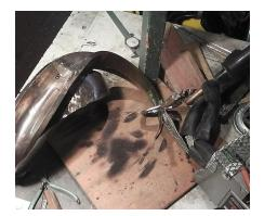
This sequence of images shows how the pits were welded. The first image shows the two pits circled in black. The second shows the 0.025" diameter pellets in place after applying flux (the stained area). The third is the result of welding these two pits.
